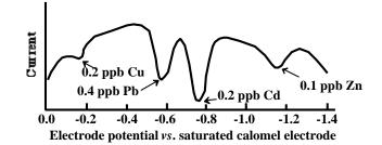
Figure 25.9 Differential-pulse anodic-stripping voltammogram of tap water at a mercury-plated, wax-impregnated graphite electrode.
