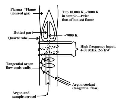
Figure 25.8 Schematic diagram showing inductively coupled plasma used for optical emission spectroscopy.
