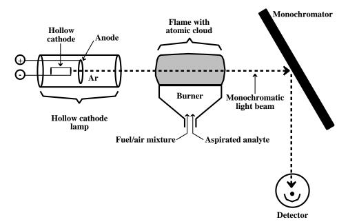
Figure 25.6 The basic components of a flame atomic absorption spectrophotometer.
