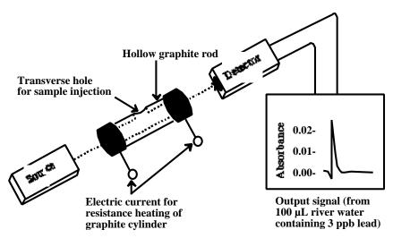
Figure 25.7 Graphite furnace for atomic absorption analysis and typical output signal.
